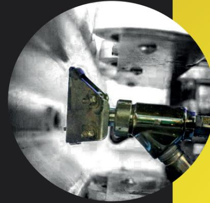
Bead gun for application of ULTRAGUARD™ microbeads
