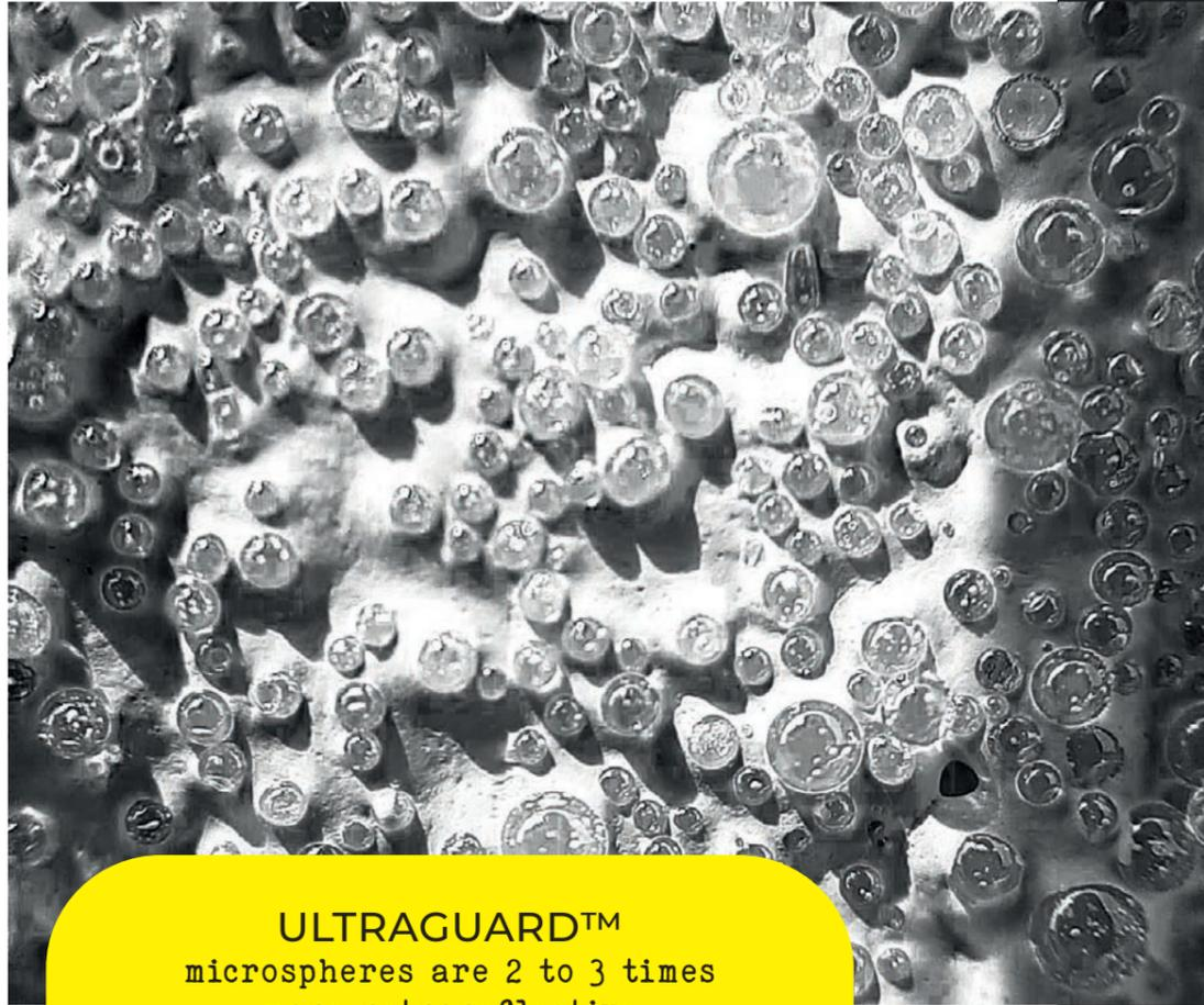
ULTRAGUARD™ microspheres are 2 to 3 times more retroreflective than conventional beads, because their refractive index is higher.
